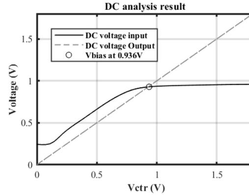
(b)  $V_{out}$  DC, sweeping  $V_{in}$  across the control range.  $V_{bias} = 0.936V \simeq \frac{AV_{DD} - AV_{SS}}{2}$
