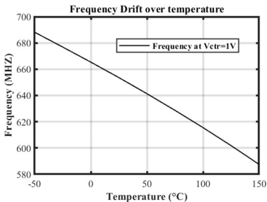
(e) Temperature performance at  $V_{ctr} = 1V$ : frequency drift of  $-0.5MHz/^\circ C$
