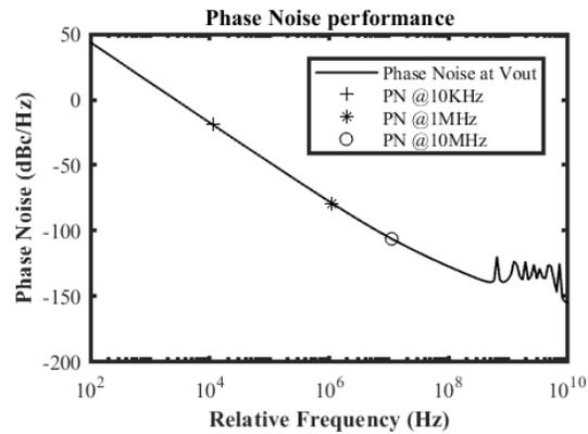
(d) Phase noise analysis: Phase Noise @ 10MHz = -105.00 dBc/Hz; Phase Noise @ 1MHz = -77.78 dBc/Hz; Phase Noise @ 10KHz = -17.80 dBc/Hz.
