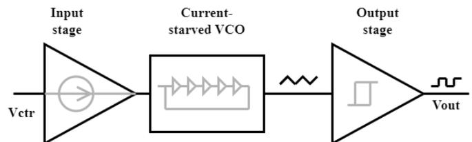
Figure 2: Circuit diagram: input stage with current linearisation, current starved ring oscillator, and output buffer with differentiation functionality
