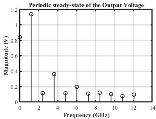
(c) Frequency spectrum of the periodic steady-state;  $H_1$  at 1.2GHz,  $H_2$  at 2.4GHz
