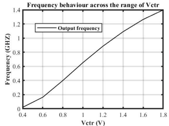
Figure 1: Complete frequency range between 20MHz and 1.4GHz, with linear behaviour across 86% of the Vctr values
